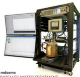
redoxme BATCH EC WATER TREATMENT TEST STATION - T, turbidity, conductivity, pH
